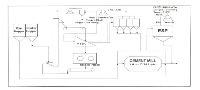
The fines classified from V-Separator are then introduced in the battery of four cyclones where solids are separated from air stream and then fed to ball mill. In order to increase the output and also at reasonable energy consumption, SCL was thought about of close circuiting the Ball mill.
