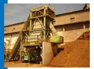
In the construction industry in Japan, wood plays a significant proportion of construction material. As the buildings are brought down and renovated, a lot of wood is available for disposal. A subsidiary company of Taiheiyo Cement Corporation purchases the wood from the demolition companies, crushes them and supplies them to the cement plant for disposal. Saitama Cement plant has installed a 50 MW capacity power plant with biomass as fuel. 50% of the power generated is exported to the grid.
