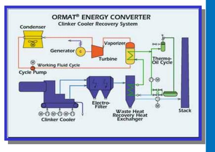
successful models have been introduced in the market. One of the most promising technologies for waste heat recovery from clinker cooler vent gases is the Organic Rankine Cycle.
