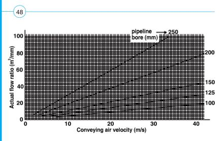
The influence of air velocity and pipeline bore on volumetric flow rate
