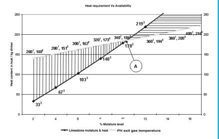
The graph gives the correlation between the heat content available (kcal / kg clinker) in the preheater gas for different preheater outlet temperatures (Deg C) and the heat required for Raw mill (kcal / kg clinker) for different lime stone moisture levels. The assumption made is the preheater gas volume is about 1.5 Nm<sup>3</sup> / kg clinker.
